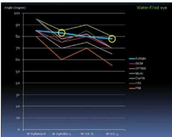
Figure 3. Semiquantitative measurements of the field angle of fundus observed through the wide-angle viewing systems in a model eye filled with water. The yellow circles indicate that the field angle of view of Resight is less influenced by pupil size than any other studied wide-angle viewing systems in the water-filled condition.
